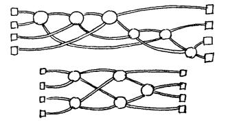
Figure 8.4: Two different networks for sorting four input values
